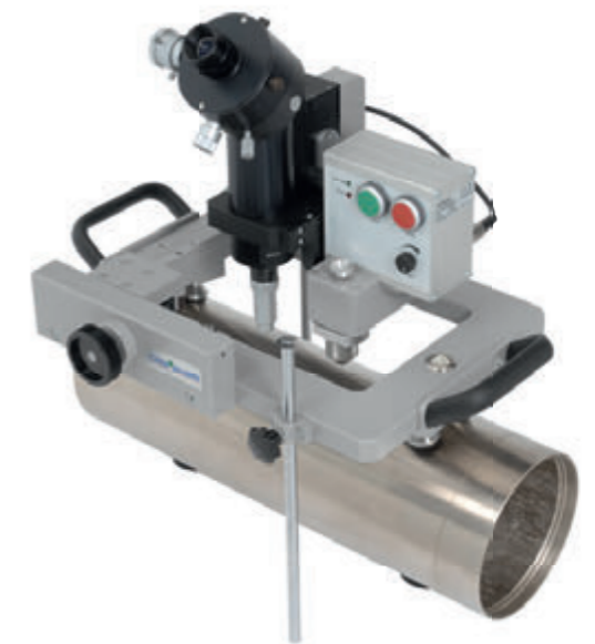
Portable Vickers HVWA 06 for hardness determination on curved surfaces
